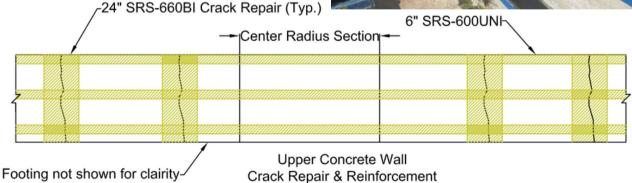
By utilizing both SRS's unidirectional and bidirectional fabrics which are bonded to the substrate with a structural epoxy adhesive, the walls were able to be repaired and reinforced against future damage. The carbon fiber reinforced polymer system (CFRP) provided permanent localized crack reinforcement as well as global strengthening of the walls. The dual component American made system has been designed by engineers and rigorously tested as permanent repair solution for these applications.
