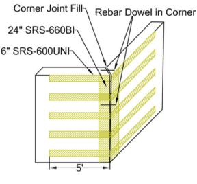
The large void in the broken corner joint was filled with a non-compressible hydraulic cement prior to the installation of the CFRP. To ensure a a flat and even profile was met beneath the carbon fiber, each mortar joint was filled flush to allow for the SRS-600 Unidirectional carbon fiber to be securely wrapped around the corner to provide global strengthening of the corner.
