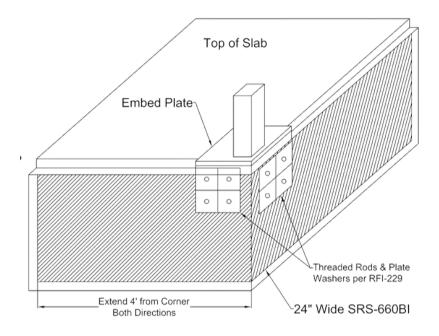
The anchors were still going to be needed but the SRS-660BI was to be installed to confine the areas and then once cured, the anchors could be drilled without worry of further cracking.
